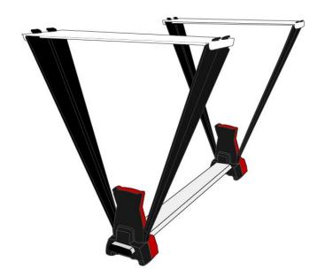
The system should mount on any standard tripod, or you can set it on a table. Make sure the red side of the sensors are facing away from the shooter. The closest sensor should be plugged into the **START** port, and the further sensor should be plugged into **STOP**.
